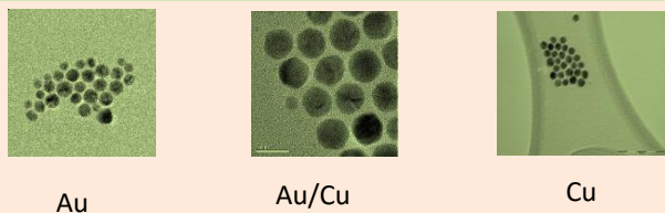
Scheme 2. HRTEM of Au (8nm), Cu (12 nm) and bimetallic Au/Cu NPs (6 nm) stabilised with decylphenyl (DP) groups.
